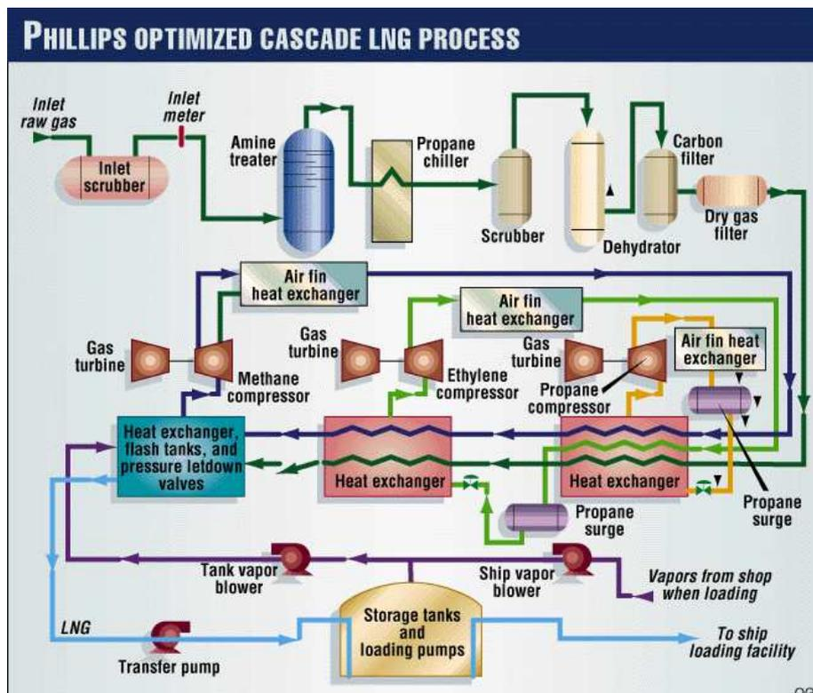
Figure 2: Phillips Optimized Cascade Process. Image from: <http://ogj.com>
