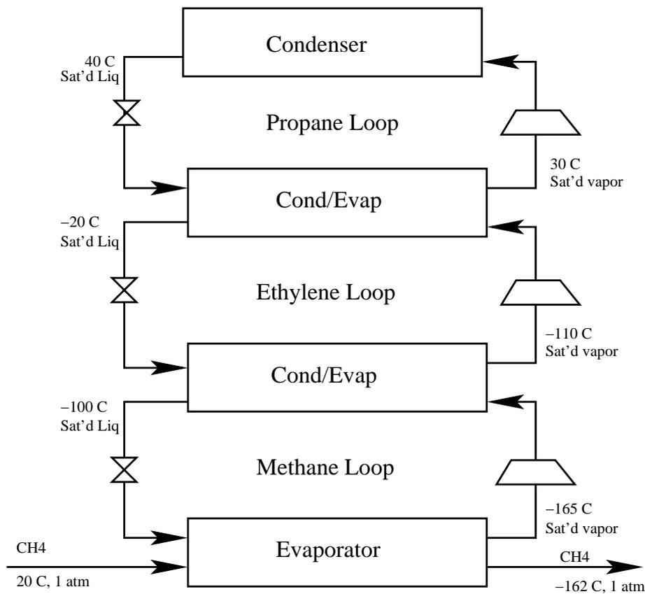
Figure 3: Base Case: simplified cascade process.
